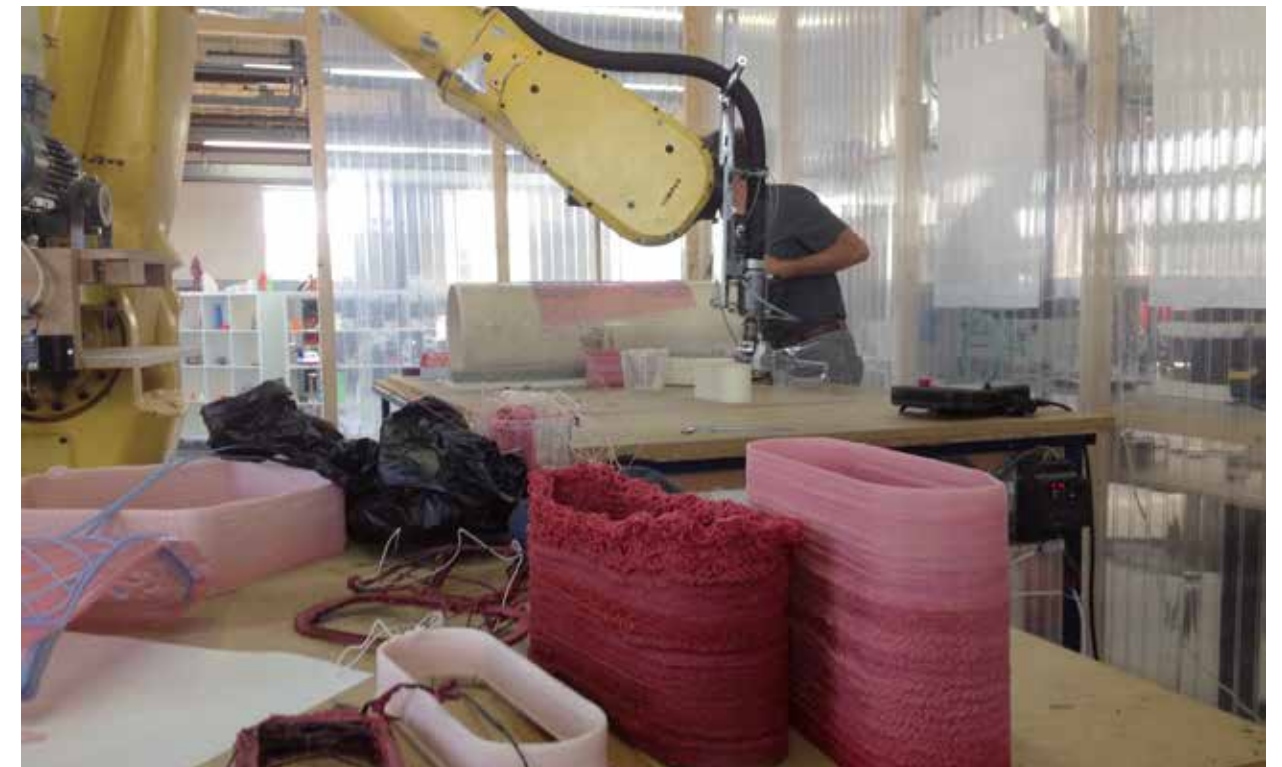
Large scale 3D Printing with an industrial robotic arm.
