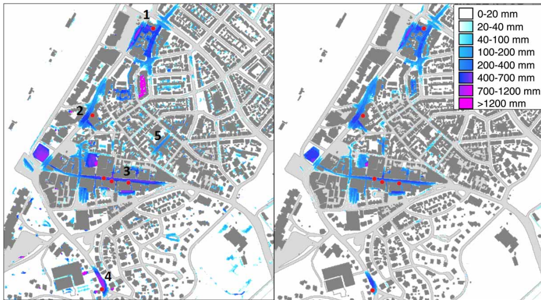
Figure 4 | Depth of water on street in the hilly area between dunes, determined by a surface flow model (left) and a coupled 1D–2D simulation model (right). The dots (shown red in the full colour version of this figure, available online at http://www.iwaponline.com/wst/toc.htm ) mark vulnerable locations known from the municipality database and the numbers in the left part of the figure correspond with the locations presented in Figure 5.
