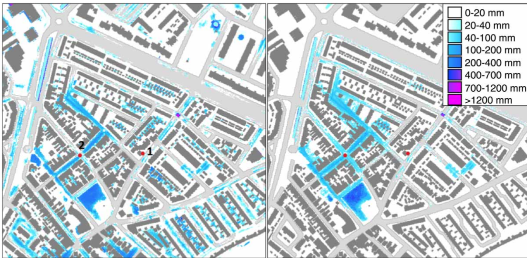
Figure 7 | Depth of water on street in the flat area, determined by a surface flow model (left) and a coupled 1D–2D simulation model (right). The dots (shown red in the full colour version of this figure, available online at http://www.iwaponline.com/wst/toc.htm ) mark vulnerable locations known from the municipality database and the numbers in the left part of the figure correspond with the locations presented in Figure 5.
