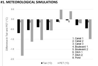
Micrometeorological simulations with Envi-met were performed to evaluate the cooling effect of eight design prototypes of Dutch urban water bodies for a hot summer day. The results in the figure above show a small or negligible cooling effect during daytime (3p.m.) - about 0.5 °C in air temperature and 1 °C in PET1 at 1.5m above the water surface - by reference to a situation without water. During nighttime (not shown), a thermal effect of the water is virtually absent.
