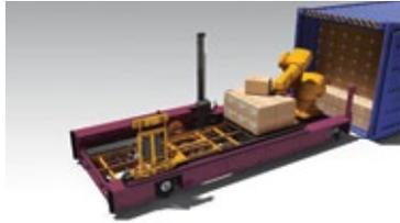
a command and the dimensions of the products it has to unload, the pIQr enters the container, using its omni-directional wheel system. When it approaches the products, it will use its vision system to size up the products, scanning it until the 3D-scan matches the dimensions it is looking for.
